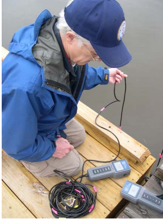
Water Quality Monitoring Coordinator Kermit Smyth practices using DO meters on the Cathance River
