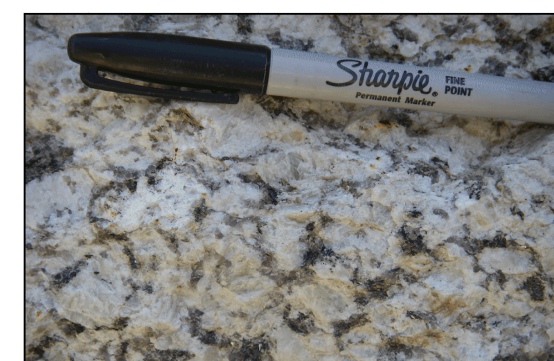
Photo 6. Representative close-up view of granite (Dg) in the Richmond quadrangle. The rock is composed primarily of cream-colored feldspar with lesser amounts of translucent gray quartz, and black biotite (mica). (Locality 6: Southwest part of the quadrangle, approximately 1500 feet northwest of the intersection of Route 24 and White Road, Bowdoinham.)
