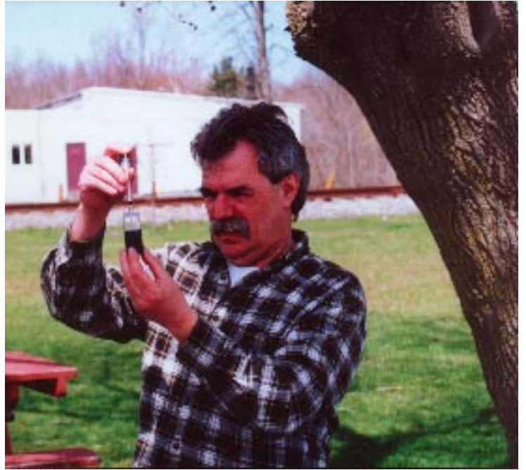
Alchemy - testing for dissolved oxygen, an indicator of water quality.
