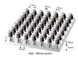
Figure 5.6 "Pelcar" concrete substrate
