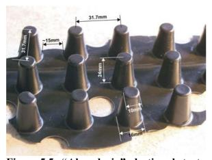
Figure 5.5 "Akwadrain" plastic substrate
