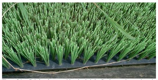
Figure 5.1 Bristle substrate with nylon bristles fixed to a polypropylene sheet
