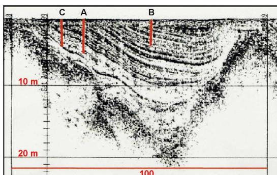
**Location 5.** Seismic section from New Meadows River. Layering in seismic image represents layering in glaciomarine deposits similar to that seen at Location 1. Location and length of cores taken from sediment are represented by the capital letters A, B, and C. The upper part of the seismic sequence is likely the distal equivalent of the sand plain. Radiocarbon-dated fossil shells from core C and core B are respectively 13,300 and 12,300 years before present (Oakley, 2001).
