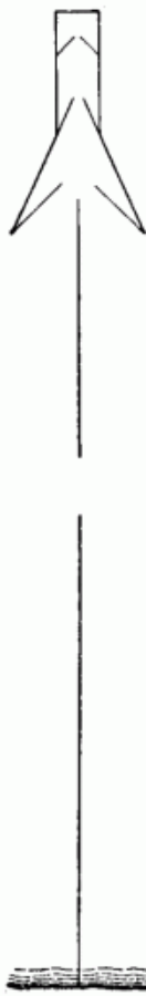
Salmon weir, Castine. —Hedge 200 feet long, made of stakes driven in mud interwoven with brush to low-water mark, covered with netting beyond. Great pound, 30 feet long, 30 feet wide at base, made of netting; entrance 8 feet wide. Inner pounds, 10 feet wide, with board floors; outer entrance 2 feet wide, inner 1 foot. Value, $70.
