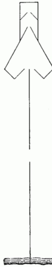
Salmon weir, Stockton. —Leader 200 feet long; brush from shore to low-water mark; remainder brush at bottom; netting at top. Head 60 feet long; outer pound 40 feet, middle pound 12 feet, inner pound 8 feet; brush below low-water line, netting above; plank floors in two smaller compartments. Value, $40.
